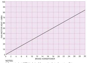
1. Fan motor heat (MBh) includes 1.1 correction factor for motor efficiency.
